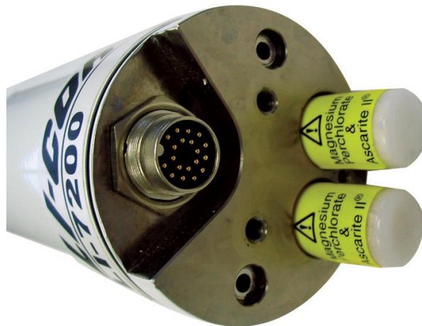
Figure 6-3. Remove the thumbscrew, thread into the bottle covers and pull straight out to access the scrubbing bottles.
